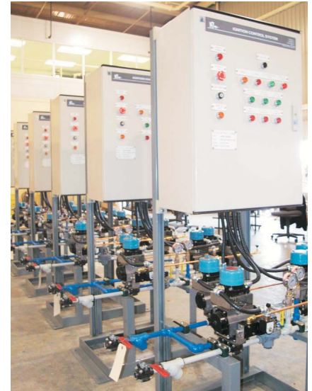
OIL IGNITOR CONTROL CABINET / VALVE TRAINS
