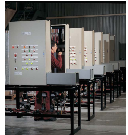
IGNITOR CONTROL CABINET/VALVE TRAIN ASSEMBLIES
